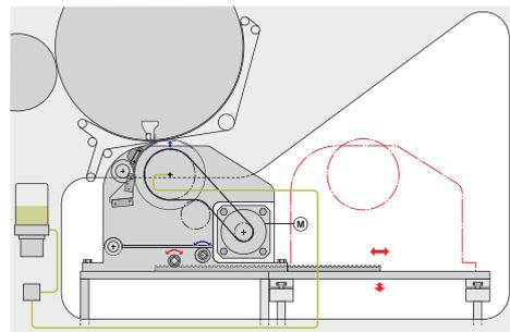
Fitting position of the cylinder stitcher with individual motor.
