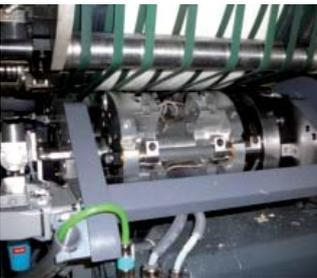
Cylinder stitcher integrated in the folder with double circumference and dedicated AC motor drive (11 millimeters and/or 16 millimeters staple sizes).
